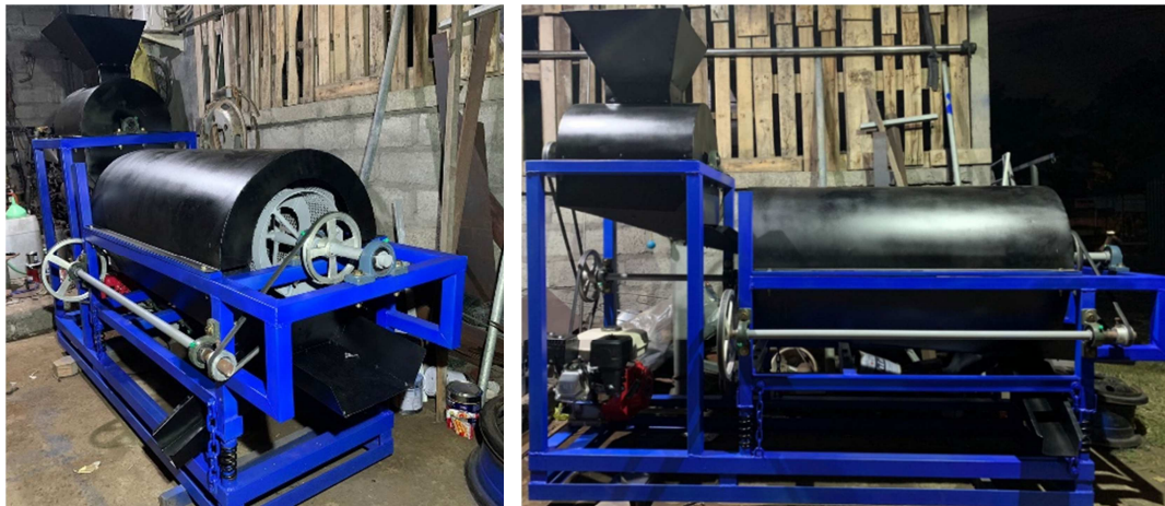
Figure 3. Clove Flower Threshing Machine Design.
